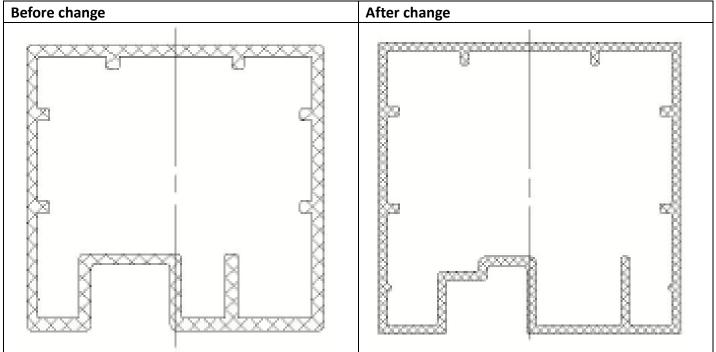
Hongfa used 2 types of tubes, the plan is it to use in future only 1 tube for the packing for HF46F. To unity tube packing and reduce tube packing type, Hongfa plans to remain 2-type tube packing type. The change has an influence to the inner structure, the length and outline dimension will not be changed
