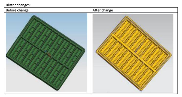
The size of the inner slots of the blister to accommodate the relay is too large and it is easy to shake the product. The relay will be now better protected in the blister, because the size of the inner groove will be reduced and the structure will be changed. The outer dimensions of the modified blister will be unchanged.
